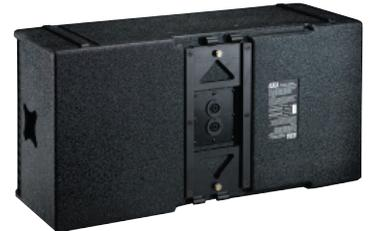
At the heart of the ExoSpine system is a rear-mounted steel track and hinge assembly. When coupling two AXIA cabinets, the hinge plates slide into position and a pin is inserted. A locking ring and cable keep the pin securely in place. During transport the hinge plates retract to a storage position. The weight of an AXIA array is supported by this steel-to-steel hinge point and will allow the flying of up to 12 AXIA cabinets in a vertical line array.
