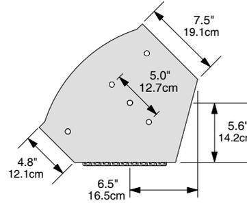
Twelve 5/16-18 threaded attachment points provided; points on 5.00-inch spacing compatible with Ultimate Support BMB-200K mounting bracket
