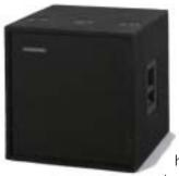
The MS18 is a specialty loudspeaker designed for output in the 35 to 140Hz range. While technically a subwoofer, it is best considered as a compact, versatile, bass reinforcement loudspeaker. The unit features a 1000 watt 18-inch woofer mounted in an easy-tohandle cube-format enclosure. The top surface of the MS18 contains three
